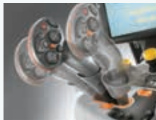
Forced based movement enables the operator to change speed and direction.
