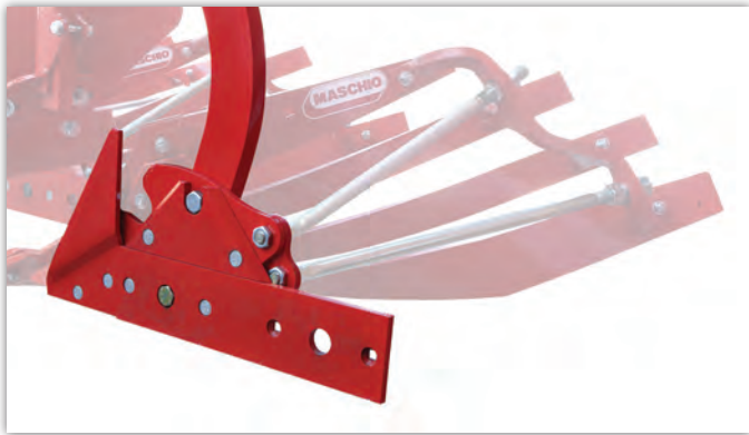
Simple body change Switching between different sizes and types of mouldboards is a straightforward operation that involves loosening a few bolts on the frog. Slatted and conventional bodies are available.
