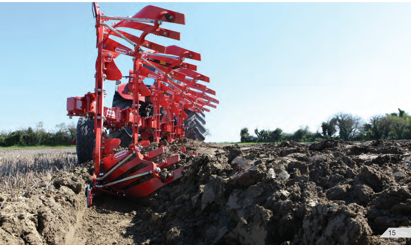
Simple body change Switching between different sizes and types of mouldboards is a straightforward operation that involves loosening a few bolts on the frog. Slatted and conventional bodies are available.
