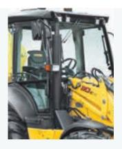
• A pillar exhaust mount for clear view of loader
