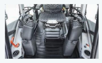
Backhoe joystick towers adjust in all directions for the most comfortable position
