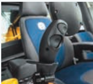
Shift button and ground speed unlock (behind)
