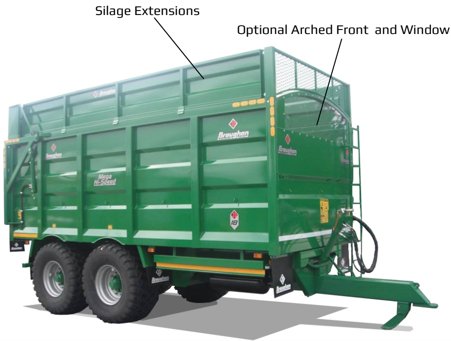
Trailers come standard with hydraulic brakes with the option of adding air or ABS brakes
