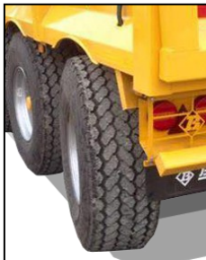
Steer Axle - available on twin axle and tri-axle trailers
