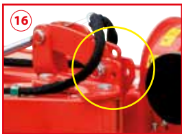
Pin safety lock for transport
